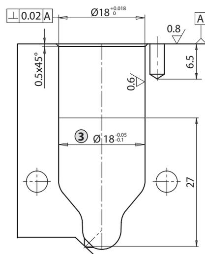
\* Gate diameter is approximate and could vary depending on injected volume and part wall thickness.
