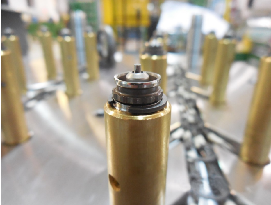
Hot half for multicavity moulds with special nozzle for rPET materials (© Thermoplay)
