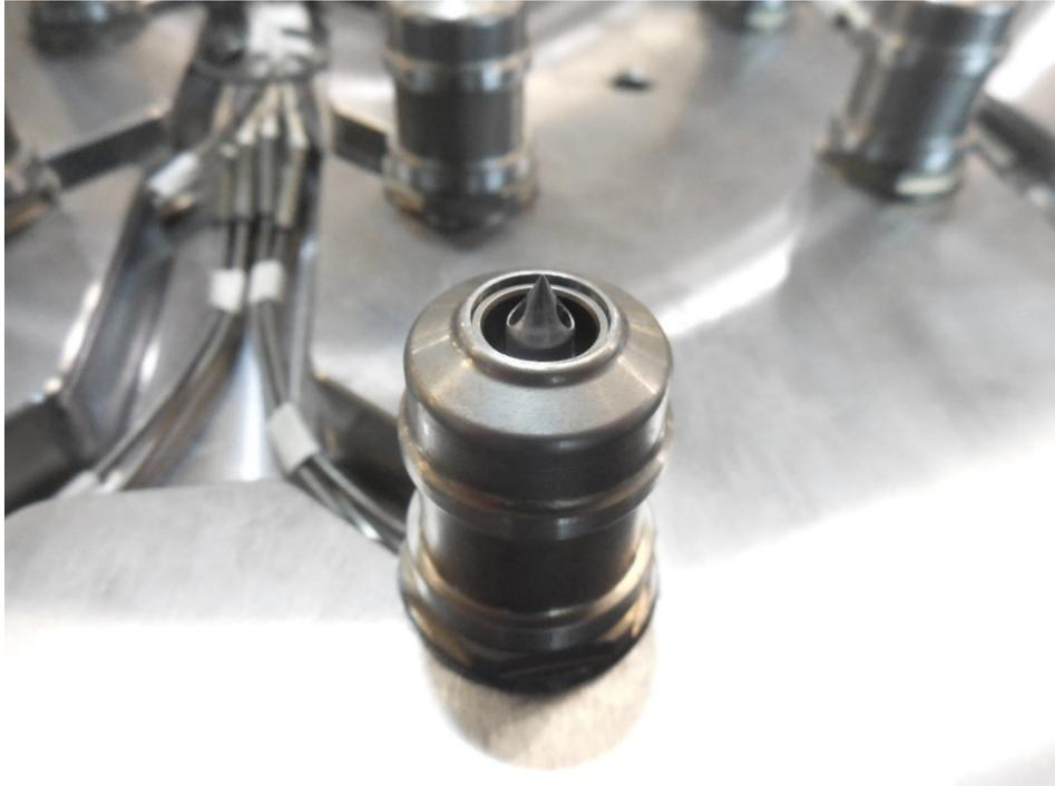
Fig 1: Thermoplay injection system with 16 TF nozzles provided with D-Bushing (© Thermoplay)
